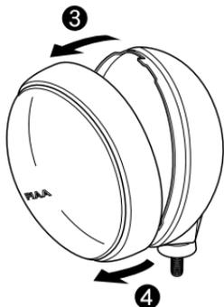
If the bulb is hot from use let it cool before touching or removing it from the lamp. To remove the main bulb (H4) unplug the socket from the back of the bulb. Release the wire retainer and pull the bulb out of the lamp. Remember to only touch the bulb by the metal base, do not touch the glass part of the bulb.
